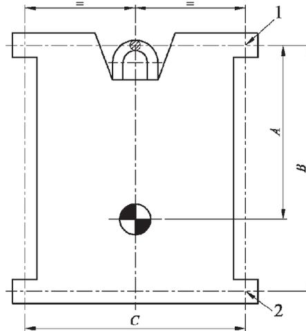
figure 14 **Acceptable forms for the means for attachment of the rope to the falling mass**
