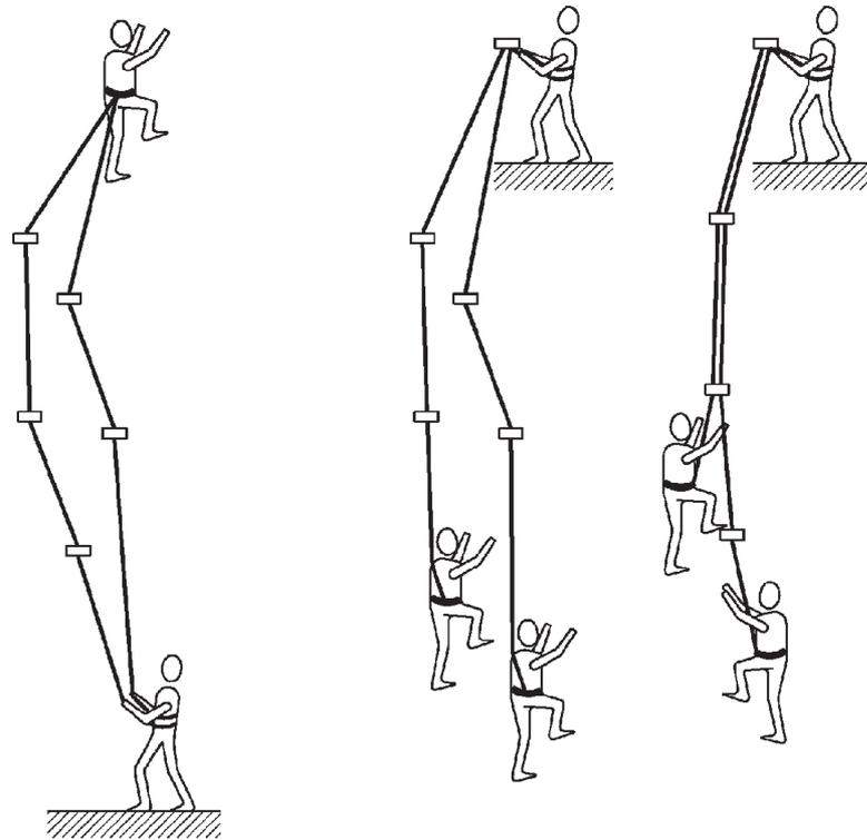
figure 2 Use of twin rope
