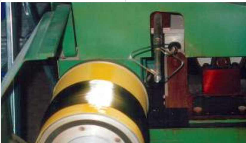
Fly ash being spun into glass fibers.
