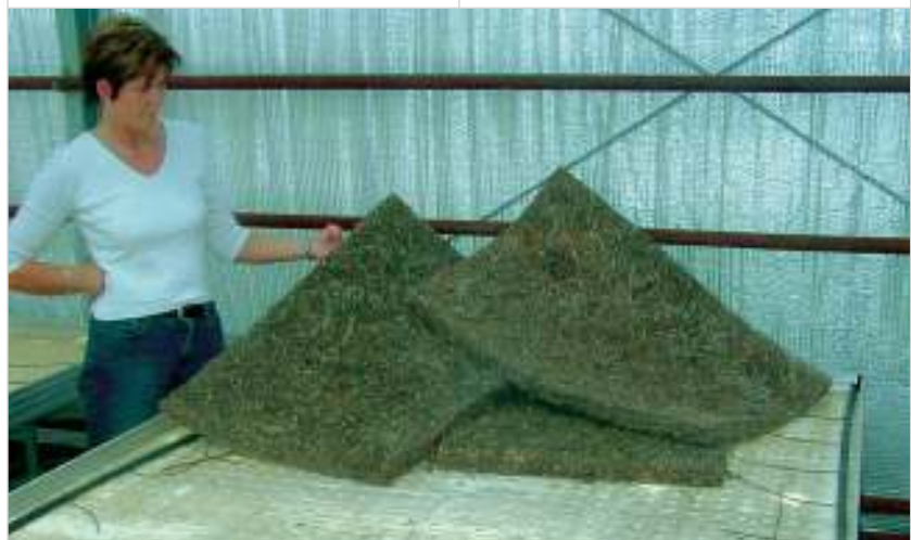
Insulation mats are one example of the many transformations of flotsam and jetsam.
