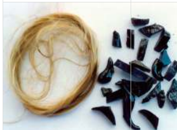
Fly ash is transformed into glass fibers to reinforce textiles, cement and plastic products.
