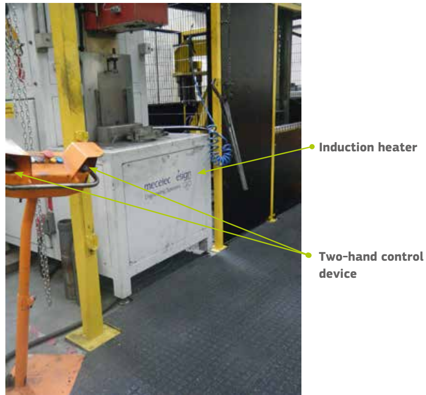
Figure 9.4 — Two-hand control device used to ensure worker separation from induction heater
