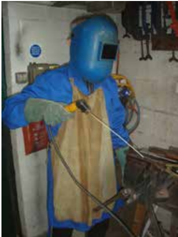
Figure 9.11 — Examples of good and bad practice in routing of arc welding cable
