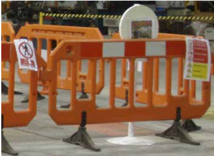
Figure 9.5 — Temporary barriers and warning signs to restrict access into strong fields generated by a temporary installation
